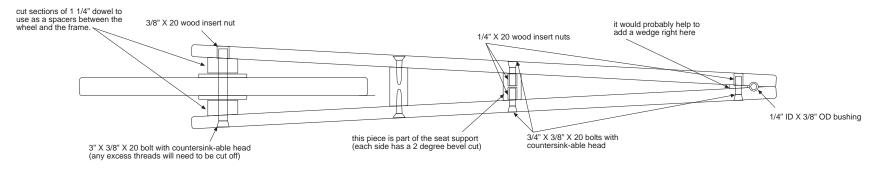
8 1/2" X 1/4" X 20 bolt (the head will be covered by the handle bar)
