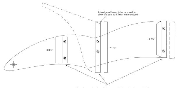
(These three wedge-shaped pieces are not in the patterns because they're essentually straight cuts with beveled edges (to match the angle formed by the two halves of the frame.)
