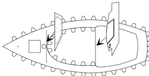
24. Lay the deck with the two bulkheads attached on the hull of the boat.
