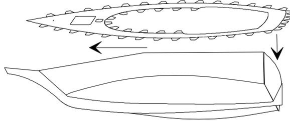
27. Gently press down on the top deck over the forward bulkhead until it touches the bottom of the boat, then glue.
